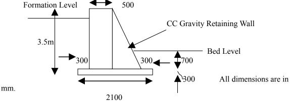
Also find out factor of safety against over turning, sliding & base pressures. Take unit wt of concrete =  $2.4t/m^3$  & unit wt of earth retained =  $1.9 t/m^3$ . Ignore wt of earth over base footing. Assume active earth pressure co-efficient = 0.3 & water table below the base of the footing. Take co-efficient of friction between soil & concrete= 0.45
